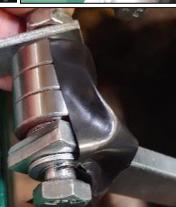
**STEP #4:** Using the 1/2" and adjustable wrenches, remove nut, belt guide, 1 x washer and 1 x bearing from idler to create space to remove belt. **TIP:** Use some tape to hold the bearing and washers together.
