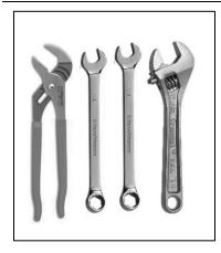
Tools: channel-lock pliers, 1/2", 7/16" and medium adjustable wrenches. Typical time to complete: 10-15 minutes. Replacement belt part number: H0705
