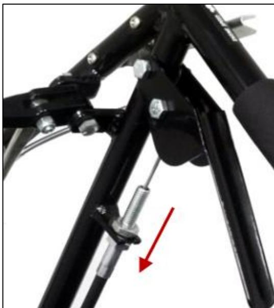
Again, the ideal function is to have firm belt tension when squeezing the lever just before it contacts the handle.
