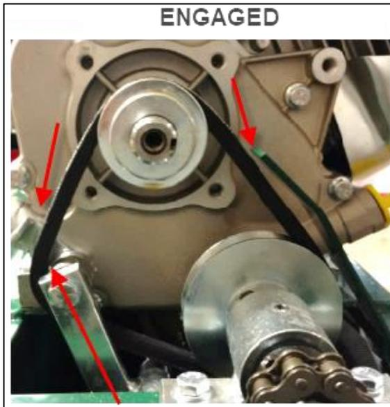
The idler position and belt engagement tension can be changed by adjusting the clutch cable. Use the lock nuts to move the outer cable in the bracket (which will move the idler position) ... downward moves the idler forward to increase the belt tension / upward moves the idler backwards to decrease the belt tension.
